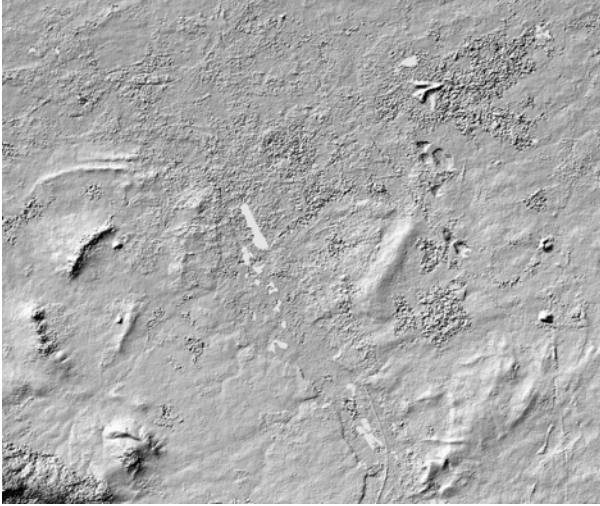
Figure 2.41 Digital elevation model derived from interferogram for the area of Hannover, Germany.
