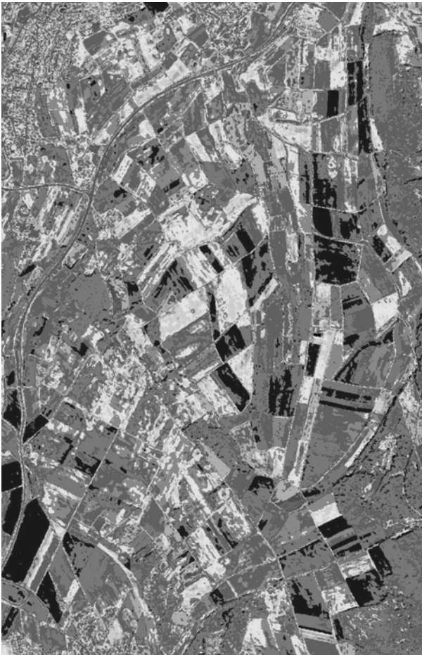
Figure 2.64 Land cover classification from a Daedalus Scanner image. Source: Daedalus, © DLR, courtesy of DLR, Oberpfaffenhofen.
