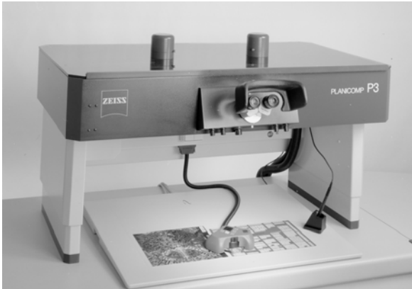
Figure 3.17 The Z/I Imaging Planicomp P3.
